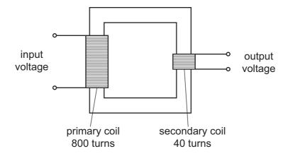
The input voltage is 240 V.
